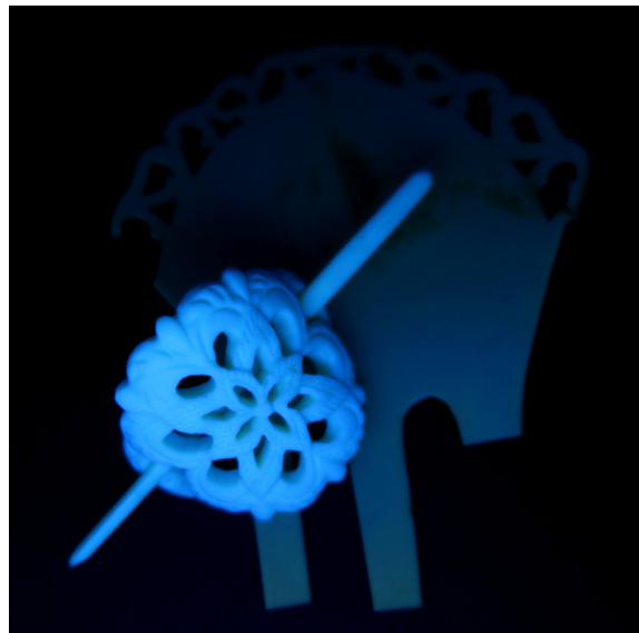
Genuine ivory is radiant when exposed to UV light, in contrast to the celluloid imitation behind it. Photograph by the author
