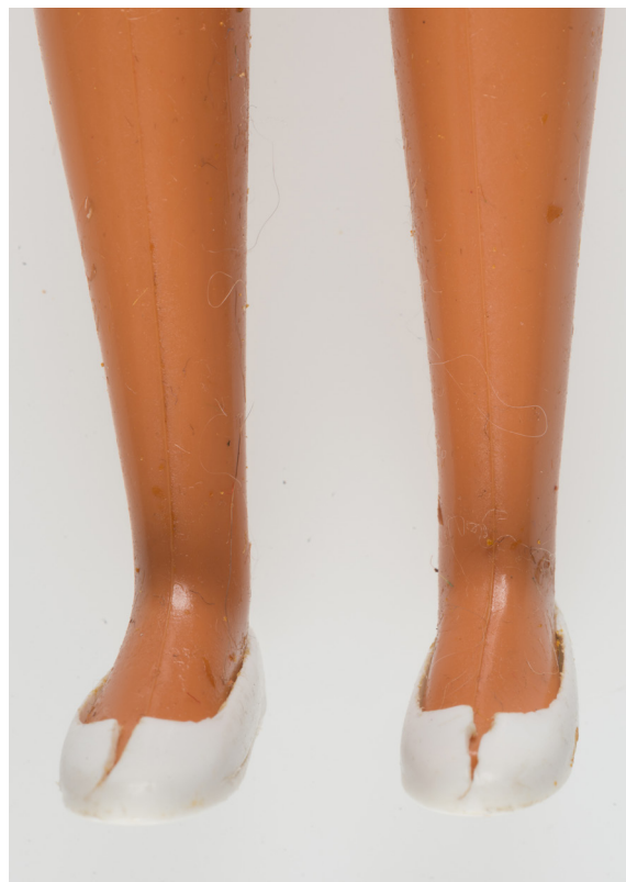
A PVC-P Barbie doll has become sticky due to plasticiser migration. Photographs: Anu Ansu and Berta Jänes. The author's collection of samples
