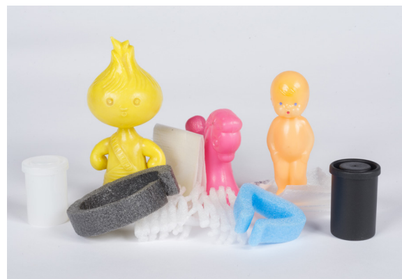
Polyethylene can be rigid or elastic, hard or soft. Photographs: Anu Ansu and Berta Jänes. The author's collection of samples
