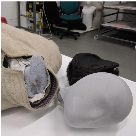
Headless horseman – polyurethane foam that has been subjected to mechanical stress. Photographs by the author
