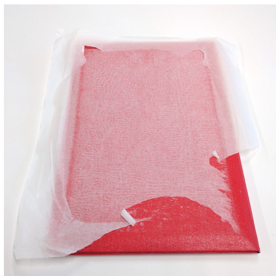
The plasticised PVC covers have become sticky and become stuck to the tissue paper used as a divider. Photograph by the author
