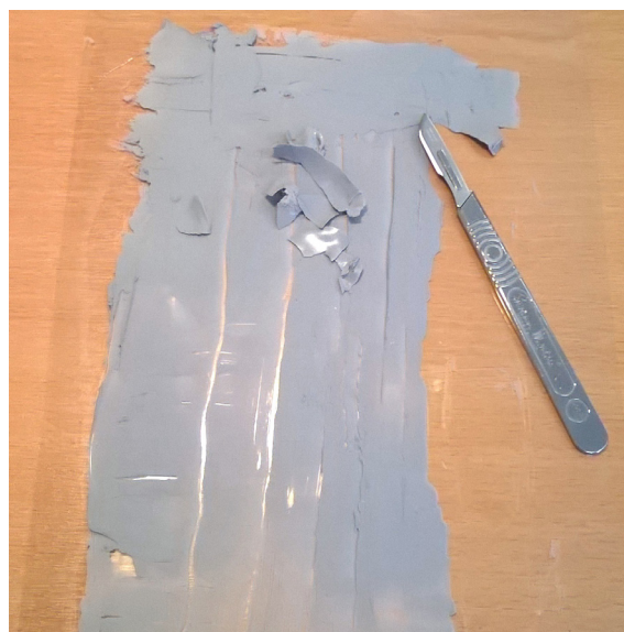
Testing of paint intended for coating display cases at the Estonian National Museum's new permanent exhibitions. After drying for a month, the paint was peeled off using a scalpel. Photograph by the author
