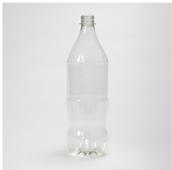
Soft drink bottles are made of polyethylene terephthalate. Photograph: Anu Ansu and Berta Jänes. The author's collection of samples
