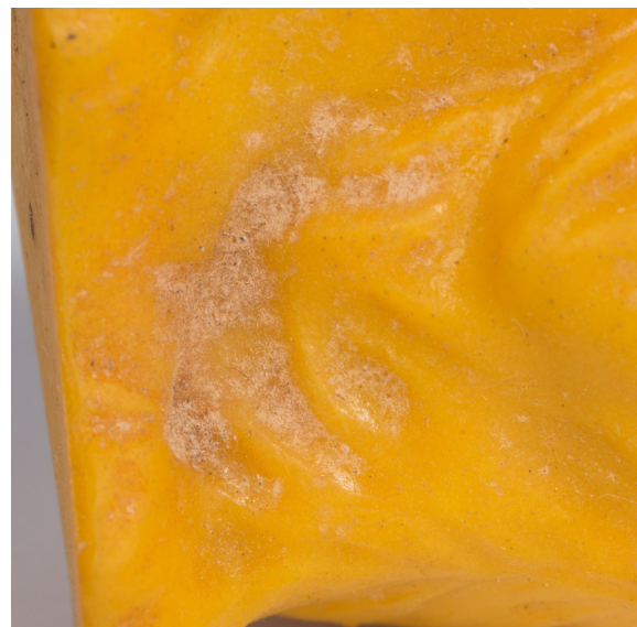
The plasticizers in PVC have migrated to the surface over time, forming a white powdery coating. Photograph: Anu Ansu and Berta Jänes. The author's collection of samples
