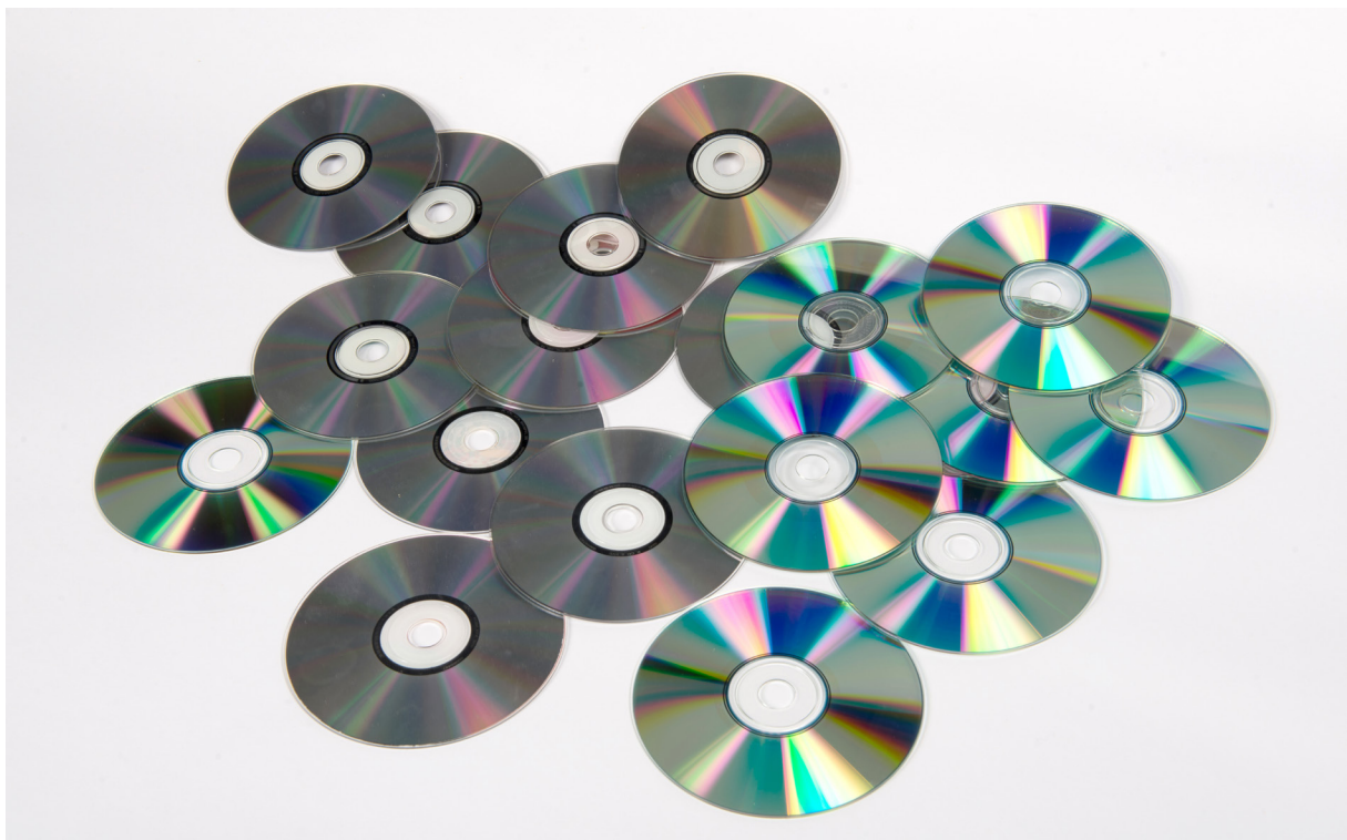
CDs are made of polycarbonate. Photograph: Anu Ansu and Berta Jänes. The author's collection of samples
