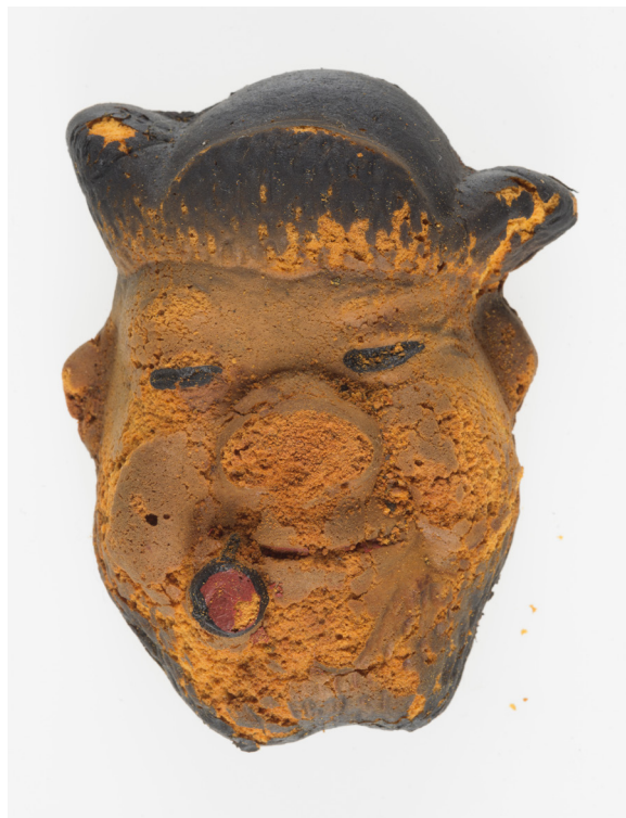
Oxidation turns foam rubber hard and very brittle over time. Photograph: Anu Ansu and Berta Jänes. ERM A 826:272
