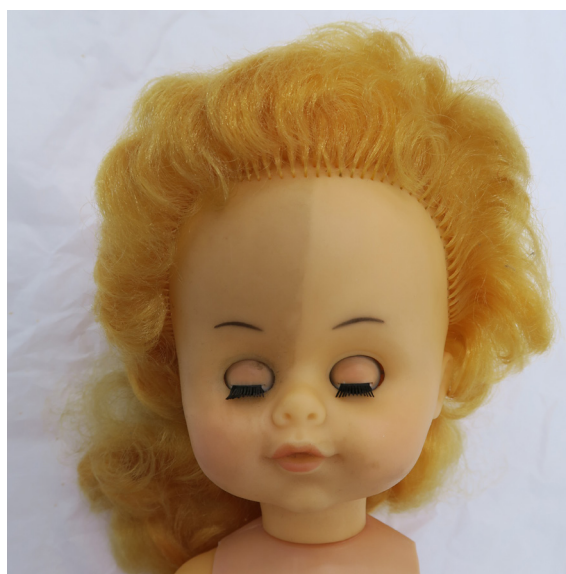
Cleaning PVC-P with ethanol. Photograph by the author
