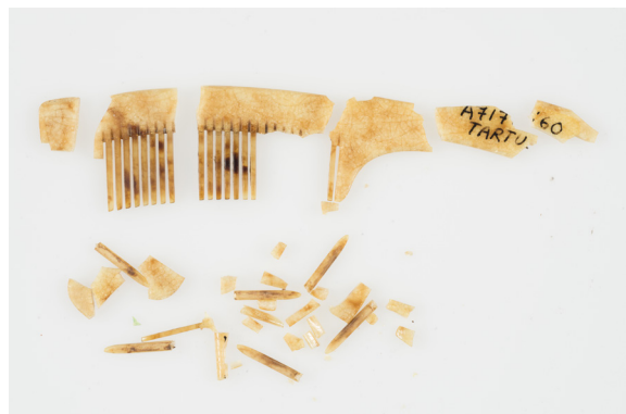
Over three years, a nitrocellulose comb has degraded visibly. Photographs: Arp Karm, Anu Ansu and Berta Jänes. ERM A 853:57
