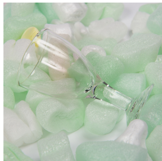
Foam “peanuts” for the safe transport of fragile items are made from extruded polystyrene (XPS) and expanded polystyrene (EPS). Photographs: Anu Ansu and Berta Jänes
