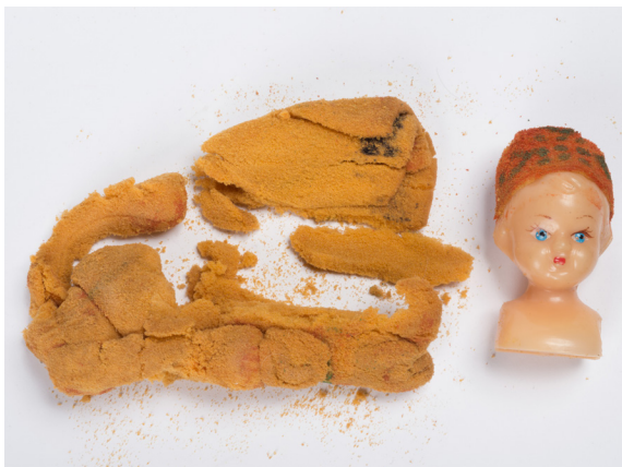
Aged polyurethane ester foam becomes sticky and collapses under its own weight. Photograph: Anu Ansu and Berta Jänes. ERM A 826:153
