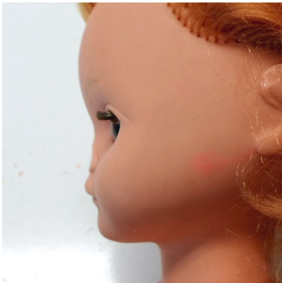
A superglue meant for PVC-P enabled repair of the damage caused by the rabbit. Photographs by the author
