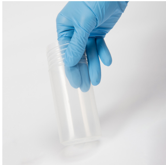
Thinner polypropylene items can be fairly transparent. Photograph: Anu Ansu and Berta Jänes. The author's collection of samples
