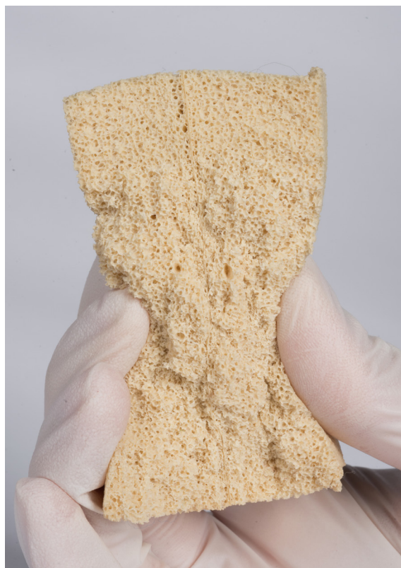
The foam rubber toy in the picture has experienced major oxidation, which turned it brittle and subject to crumbling at the slightest touch. The original colour of the fresh foam rubber can be seen in the image on the right. Photographs: Anu Ansu and Berta Jänes. The author's collection of samples
