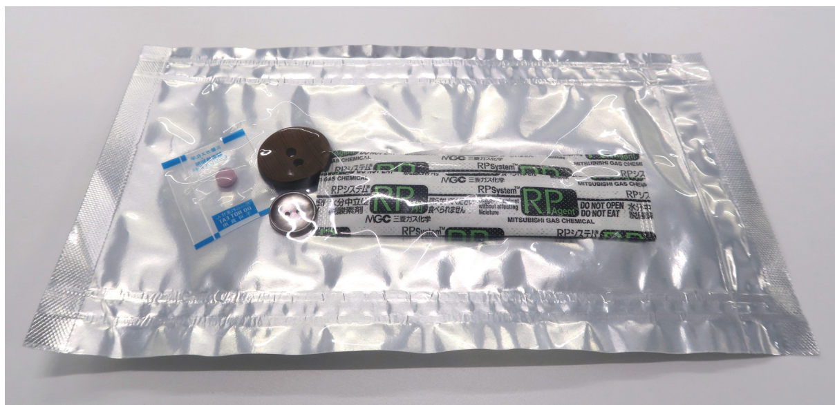
An example of an oxygen-free preservation method. A silvery opaque film (Marvelseal) and a special gas-impermeable film (Escal) were used. In addition to the Ageless packet, an Ageless Eye was also placed inside the packaging. Photograph by the author
