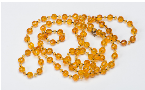
Imitation amber pearls made of glass and polystyrene. Photographs: Anu Ansu and Berta Jänes. The author's collection of samples
