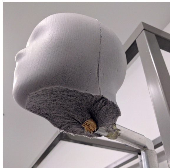
Headless horseman – polyurethane foam that has been subjected to mechanical stress. Photographs by the author
