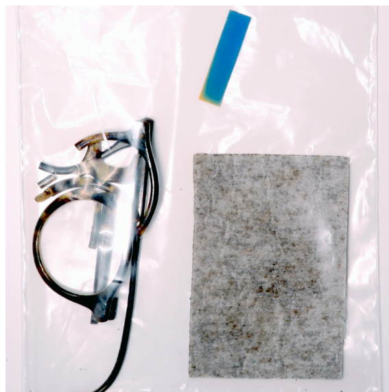
A test for determining the suitable size of a textile filter. The photograph was taken after 48 hours had elapsed. Although the sample was not large enough, the filter does clearly work when the test result is compared to a control where a charcoal filter was not used
