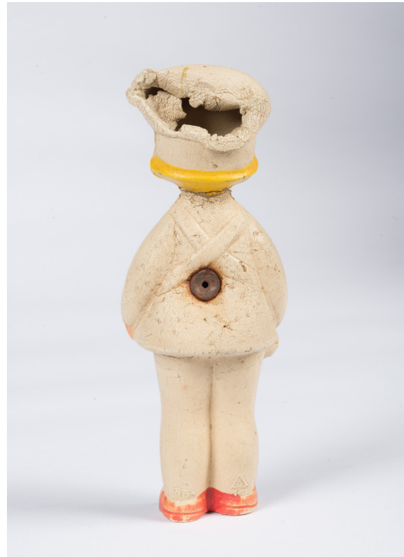
A plastic item that appears to be in good condition may in fact be severely damaged. In the photo, the rubber figure has been degraded by oxidation. Photographs: Anu Ansu and Berta Jänes. The author's collection of samples
