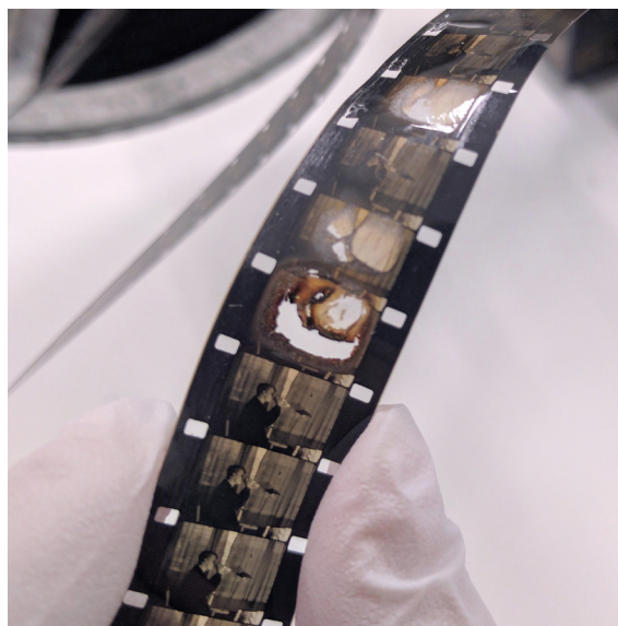
Leave a reel of film with the lamp on and the film will sustain local thermal damage. In this case, the material was cellulose acetate. Had it been a reel of nitrocellulose film, it would have caught fire. Photograph by the author
