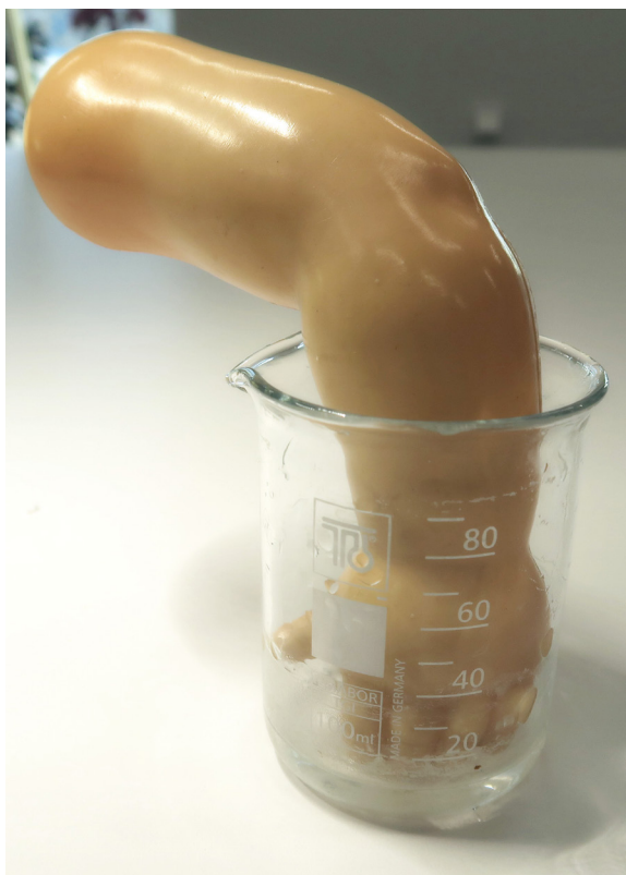
The arm of the doll (nitrocellulose) was dipped in acetone for 30 seconds and sustained severe solvent damage. Photographs by the author
