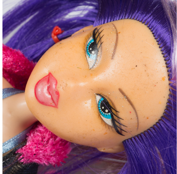
Plasticised PVC that has become sticky. Photograph: Anu Ansu and Berta Jänes. The author's collection of samples
