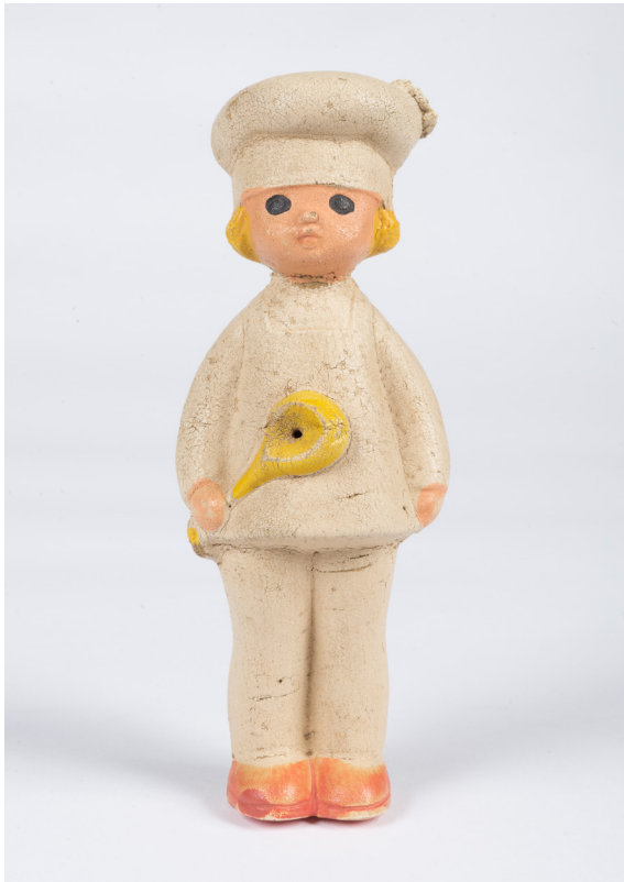
A plastic item that appears to be in good condition may in fact be severely damaged. In the photo, the rubber figure has been degraded by oxidation. Photographs: Anu Ansu and Berta Jänes. The author's collection of samples
