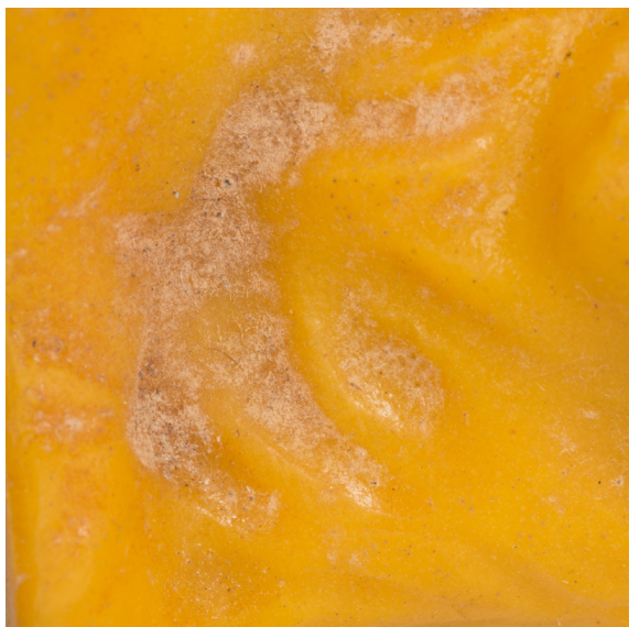
A crystallised layer of lubricant has formed on the surface of this plasticised PVC item. It can easily be removed by wiping. Photographs by the author
