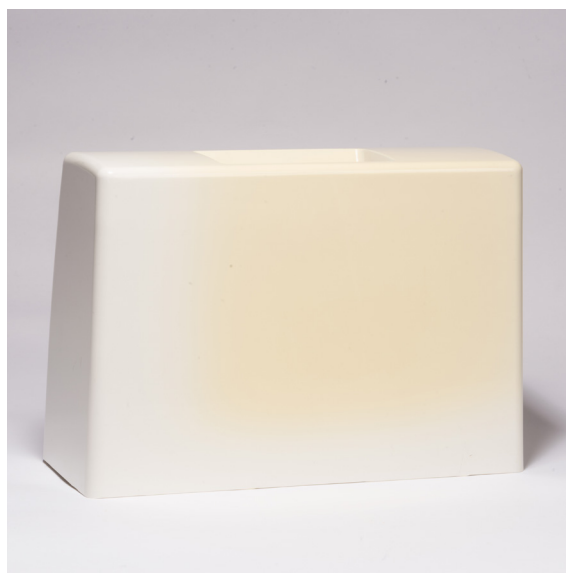
It is clear which parts of the sewing machine cover (polystyrene) have had the most exposure to direct sunlight. Photograph: Anu Ansu and Berta Jänes
