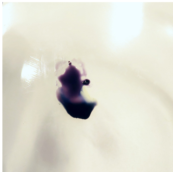
Dip test. Initially green in colour, the reagent turns lilac after a short period of time when exposed to nitrocellulose. Photographs by the author
