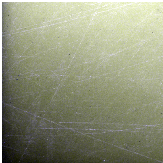
Some plastics like polyethylene are sufficiently soft to be scratched by fingernails. Photographs taken under a microscope show the same location before and after. Photographs by the author
