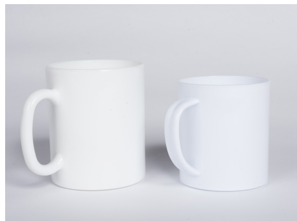
Two ostensibly similar mugs. The left one is ceramic, the right one is plastic. Photographs: Anu Ansu and Berta Jänes. The author's collection of samples
