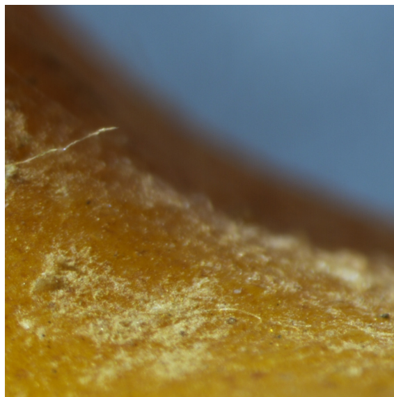
A crystallised layer of lubricant has formed on the surface of this plasticised PVC item. It can easily be removed by wiping. Photographs by the author
