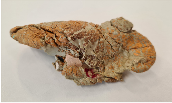
As a result of oxidation, the material properties of the natural vulcanised rubber have changed. Consequently, the rubber appears as though it has melted, and the material has become partially sticky at room temperature. Photograph by the author
