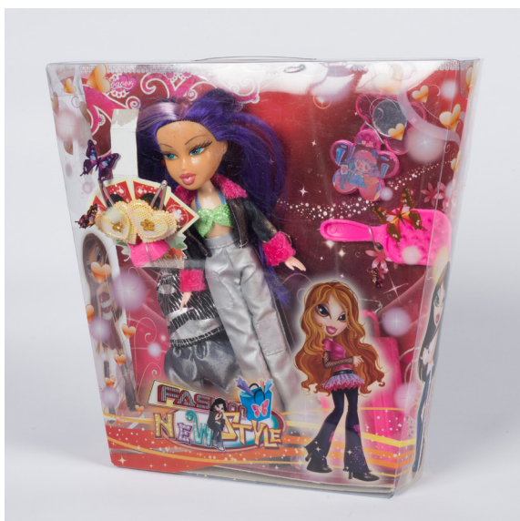
A never-used doll still in its original packaging gradually experienced chemical aging. The plasticised PVC head has become sticky due to the plasticisers migrating to the surface. Photographs: Anu Ansu and Berta Jänes. The author's collection of samples
