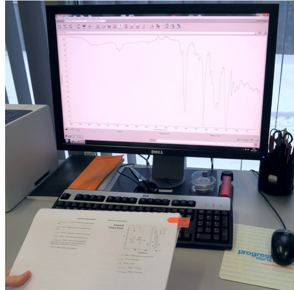
To compare the test results, the spectrum obtained from FTIR analysis is compared to spectra in a database. This requires experience and a large set of data. Photograph by the author
