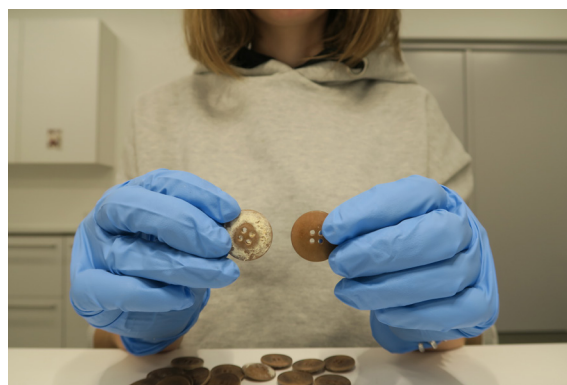
Using ethanol to clean mould from casein formaldehyde buttons. Photograph by the author
