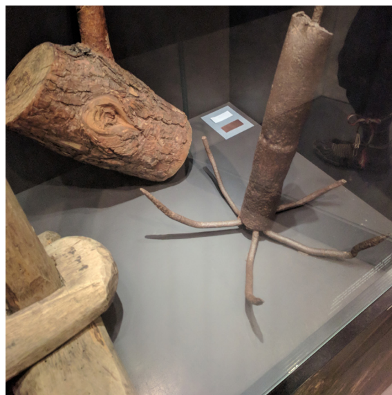
Metal coupons placed in the National Museum's Echo of the Urals exhibition display case. The lead sample became light-grey in a few months, showing that there is a ventilation problem – the aldehyde concentration inside the case is too high. The copper sample has not experienced change, showing that the concentration of chlorides, oxides and sulphur compounds is not excessive. Photograph by the author
