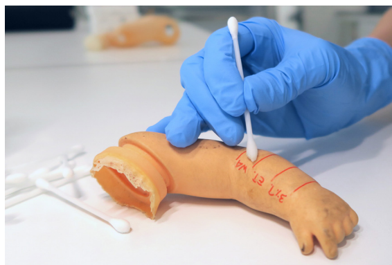
The procedure for the PVC-P cleaning test. A 1% aqueous solution of Orvus WA Paste yielded the best result, and 3% triammonium citrate and 96% ethanol also performed passably. Photograph by the author
