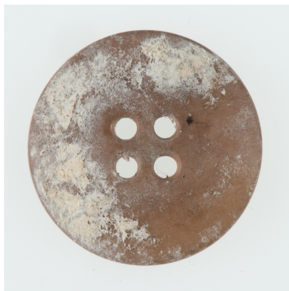
Buttons made of casein formaldehyde have mildewed in a warm and humid environment. Photograph: Anu Ansu and Berta Jänes. ERM A 984:86
