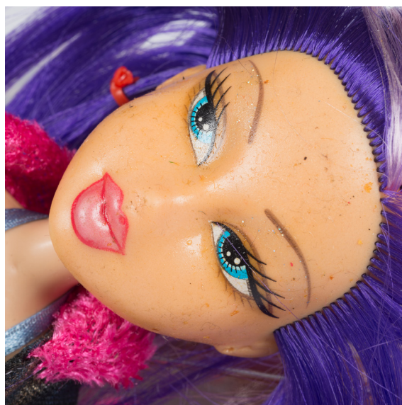
A never-used doll still in its original packaging gradually experienced chemical aging. The plasticised PVC head has become sticky due to the plasticisers migrating to the surface. Photographs: Anu Ansu and Berta Jänes. The author's collection of samples
