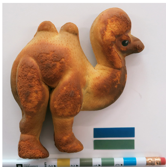
An aging rubber object gives off plentiful sulphur-containing compounds, as attested to the colour change in the indicator strip. ERM A 826:340. Photograph by the author
