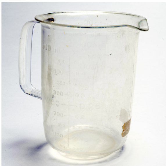
The first time it was washed in a laboratory dishwasher, a polystyrene measuring cup was deformed with stress fractures that clouded the otherwise transparent plastic. The wash cycle was at 90 °C while polystyrene melts at 100 °C. Photographs: Anu Ansu and Berta Jānes. The author's collection of samples
