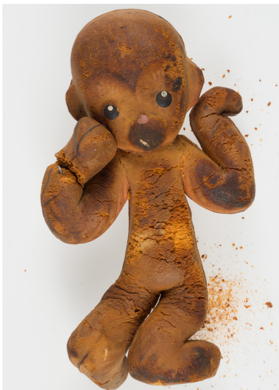
The foam rubber toy in the picture has experienced major oxidation, which turned it brittle and subject to crumbling at the slightest touch. The original colour of the fresh foam rubber can be seen in the image on the right. Photographs: Anu Ansu and Berta Jänes. The author's collection of samples
