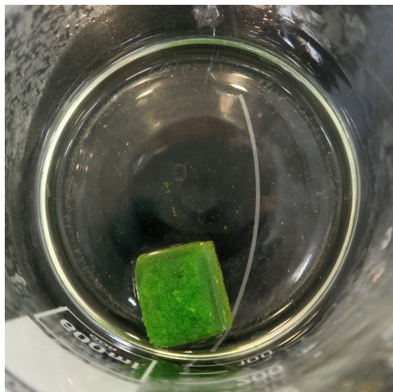
Polyurethane ether remained unchanged even after 20 minutes of boiling
