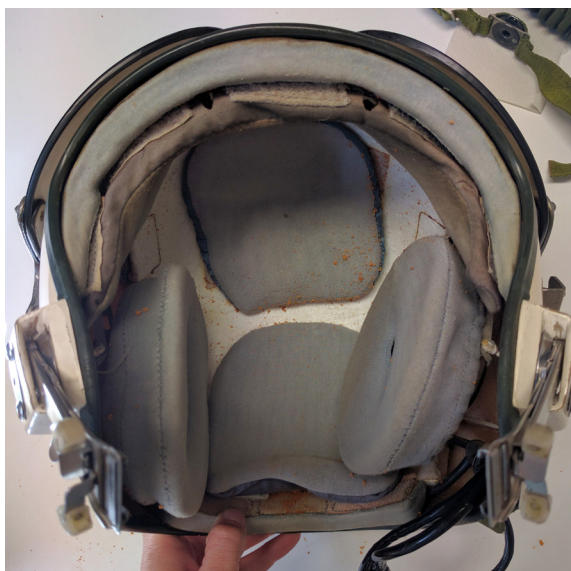
Polyester-based polyurethane foam was used as a padding material in a Soviet-era aviation helmet. Over time, it has become crumbly and sticky due to hydrolysis. Photographs by the author
