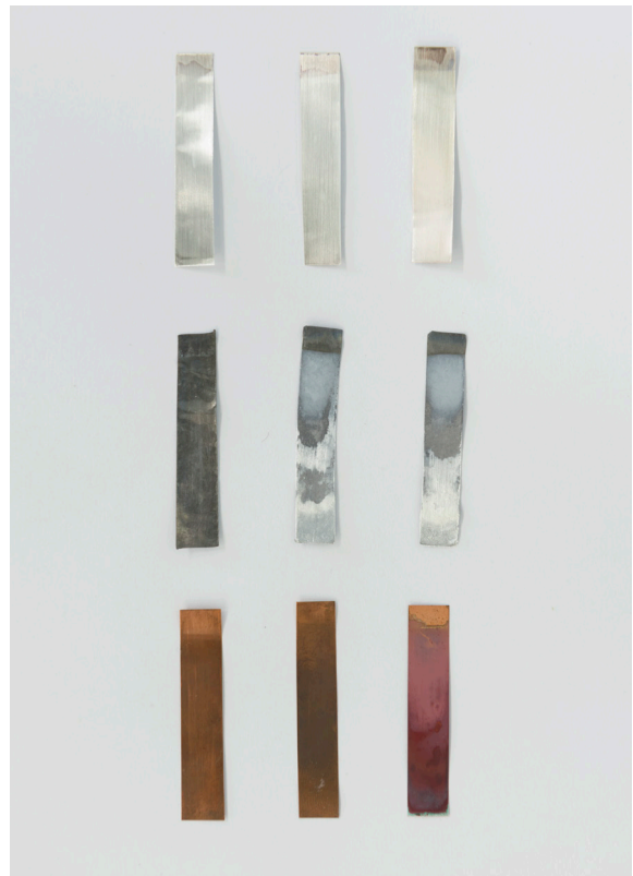
Test results. From top to bottom, these are silver, lead and copper samples. Negative control test results are shown in the left column, while the right column shows positive controls and the middle column indicates results for the sample being tested. The test confirmed that the proposed aldehyde-based paint was unsuitable for use in a sealed display case. Photographs: Arp Karm
