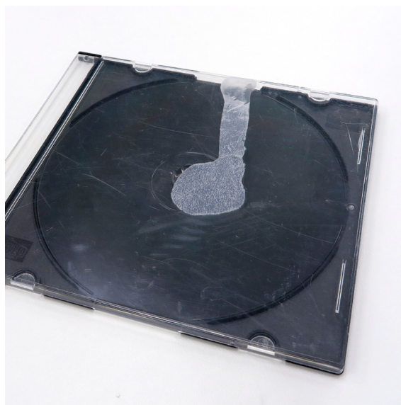
Acetone dripped on the surface of the CD-case (polystyrene) has caused irreversible damage. Photograph by the author
