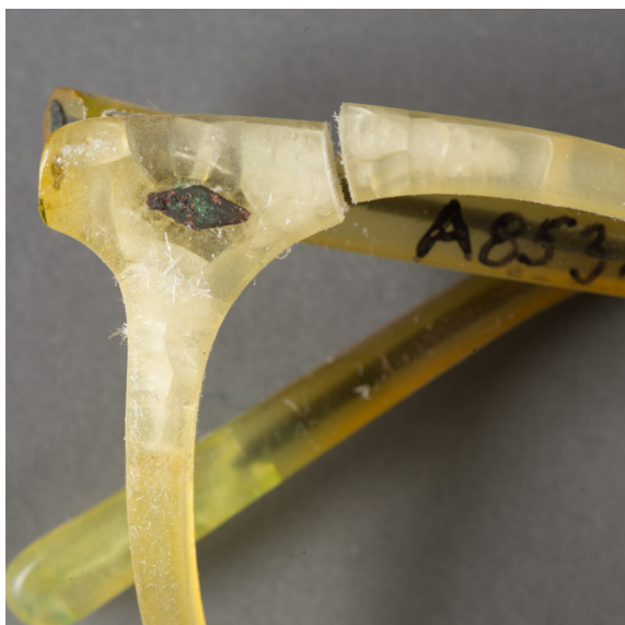
Nitrocellulose crystallised as a result of hydrolysis. Photograph: Anu Ansu and Berta Jänes. ERM A 853:57
