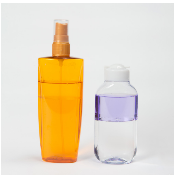
Transparent packaging and bottles for cosmetics are mostly made of polyethylene terephthalate. Photograph: Anu Ansu and Berta Jänes. The author's collection of samples
