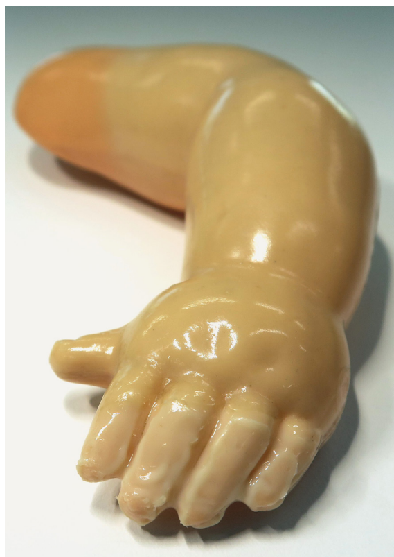
The arm of the doll (nitrocellulose) was dipped in acetone for 30 seconds and sustained severe solvent damage. Photographs by the author
