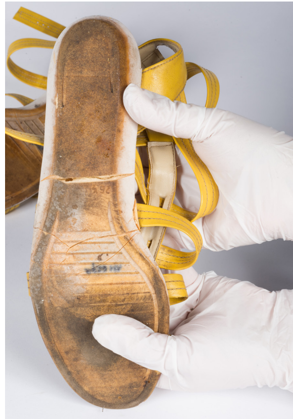
An evaluation of the condition of plastic items requires knowledge of the causes of specific damage. In this case, shoe soles made of elastic polyurethane have become brittle so they break when bent. The surface has also become sticky, showing advanced chemical degradation leading to mechanical damage. Photograph: Anu Ansu and Berta Jänes. The author's collection of samples
