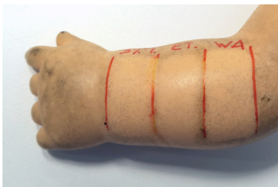
The PVC-P cleaning test shows how even the best method leaves black specks on the surface. The dirt has “seeped” into the material and can only be removed with more aggressive solvents, such as acetone. Acetone however damages PVC-P surfaces. Photograph by the author
