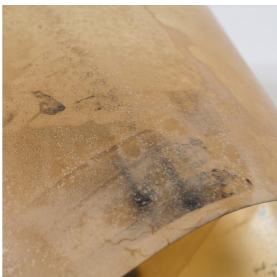
A layer of mould has formed on nitrocellulose film stored in damp conditions, damaging the footage. Photographs: Anu Ansu and Berta Jänes
