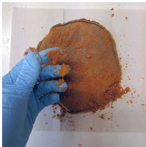
Polyester-based polyurethane foam was used as a padding material in a Soviet-era aviation helmet. Over time, it has become crumbly and sticky due to hydrolysis. Photographs by the author
