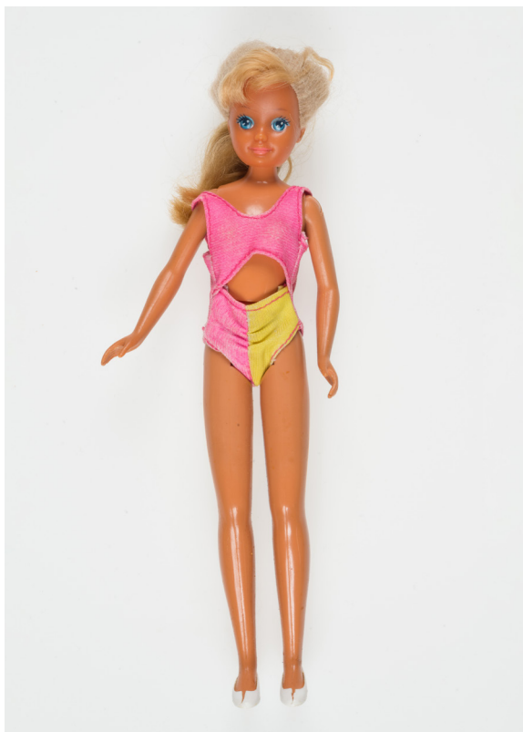
A PVC-P Barbie doll has become sticky due to plasticiser migration. Photographs: Anu Ansu and Berta Jänes. The author's collection of samples
