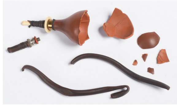
As a result of oxidation, a rubber pump became brittle, much like unfired pottery. This could have been prevented by storing it in a low-oxygen environment. Photograph: Anu Ansu and Berta Jänes. ERM AM 100:1
