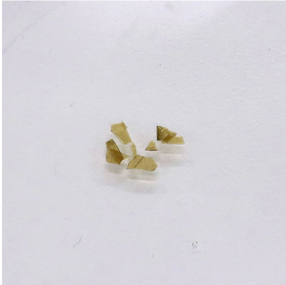
Dip test. Initially green in colour, the reagent turns lilac after a short period of time when exposed to nitrocellulose. Photographs by the author
