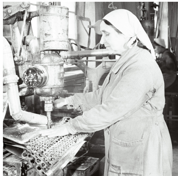
Stamping button blanks in 1948. Photograph: V. Samussenko. EFA.204.0-1790
