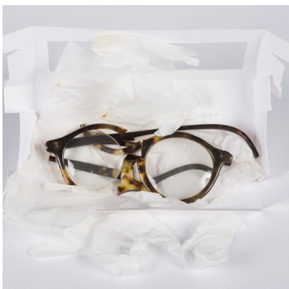
The nitrocellulose frames have become fragile in the course of hydrolysis. The silk paper used for preservation became acidic and very brittle over just a few years due to the nitric acid emitted. Photograph: Anu Ansu and Berta Jänes. ERM A 816:6
