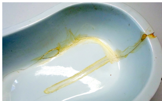
Polyurethane adhesive was used to glue together a ceramic bidet. As we see, it has become yellowed. Photograph by the author
