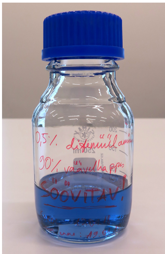
Diphenylamine reagent. Labelling should specify that it contains corrosive sulphuric acid! Photograph by the author
