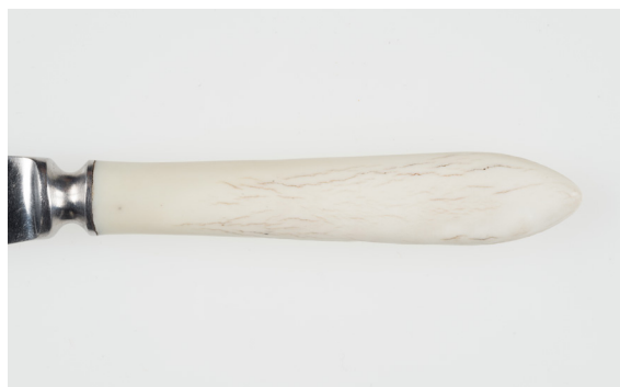
The handle of a knife made of melamine formaldehyde has been damaged by repeated exposure to water. Photograph: Anu Ansu and Berta Jänes. The author's collection of samples
