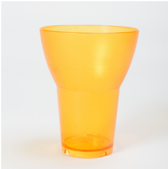
Container made of styrene acrylonitrile resin. Photograph: Anu Ansu and Berta Jänes. The author's collection of samples
