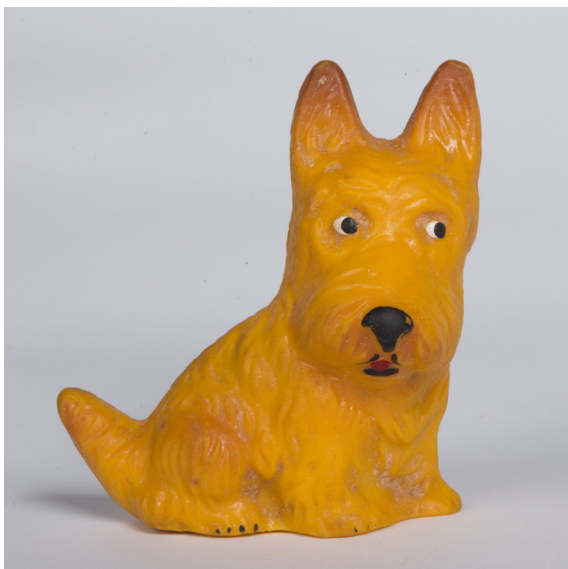
The plasticizers in PVC have migrated to the surface over time, forming a white powdery coating. Photograph: Anu Ansu and Berta Jänes. The author's collection of samples
