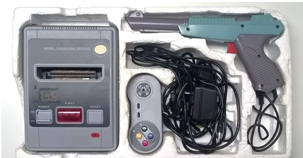
A video game console from the 1990s was stored in its original packaging. Over time, the PVC-P-coated cords deformed the styrofoam. Photograph by the author. ERM A 951:116
