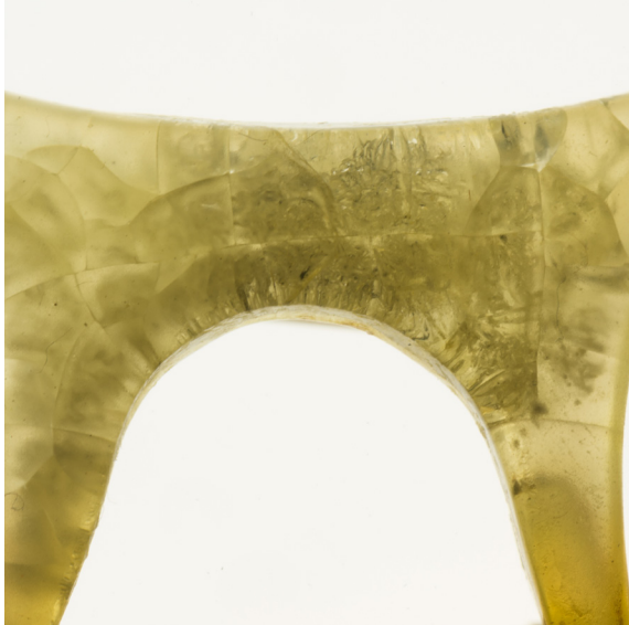
Heavily aged nitrocellulose. Photograph: Anu Ansu and Berta Jänes. The author's collection of samples
