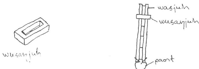
Figure 2. A leveller of barn wall boarding (EA 148: 24).
